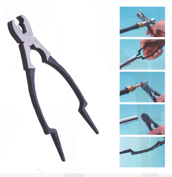
Cleaner Pliers for CO2, fully automatic and semi-automatic welding machines. Convenient for robot welding machines, such as pulling out and cutting wires, attching and detaching tips and nozzles, simultaneously removing internal and external spatter, and attching and detaching insulating tubes. Easy-to-hold uneven grip.
