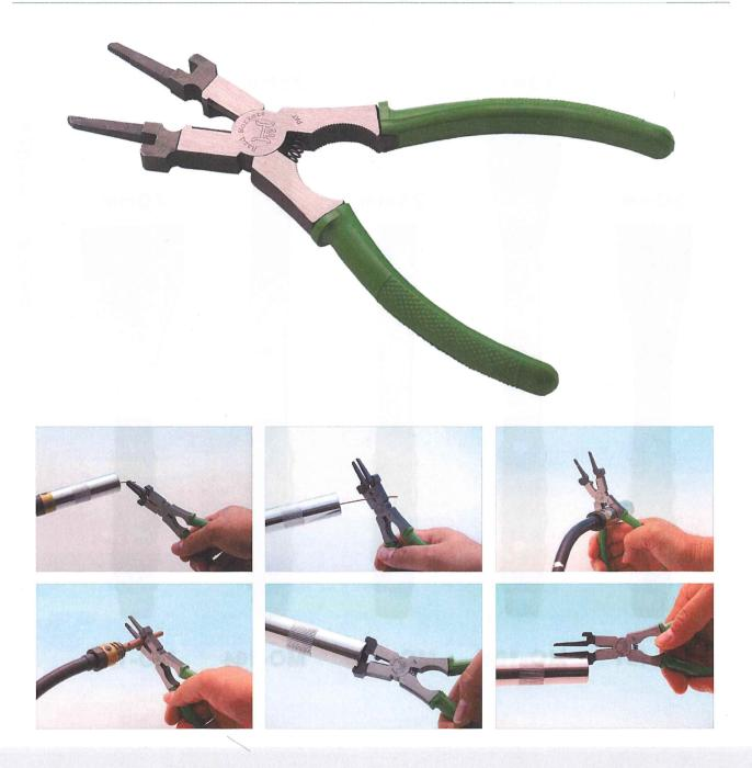
Pliers exclusively for CO2 semi-automatic welding machines. Ideal for pulling out and cutting wires, attaching and detaching nozzles, insulation tubes, tips simultaneously removing internal and exernal spatter, and removing nozzle tips and external spatter. Can cut stainless steel wires.
