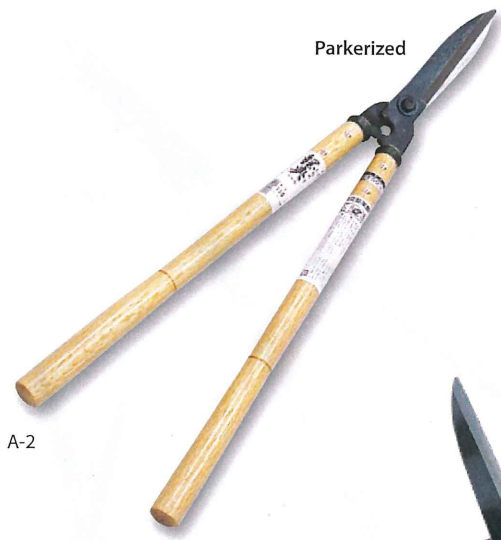
A-2 Yasuki-Hagane Clad Steel Hedge Shears Forged ■ Blade length: 150mm, Grip: 450mm ■ Weight: 895g, OAL: 650mm ■ Material: Yasugi-Hagane+Cutlery Carbon Steel Grip: Oak
