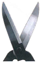
A-2 Yasuki-Hagane Clad Steel Hedge Shears Forged ■ Blade length: 150mm, Grip: 450mm ■ Weight: 895g, OAL: 650mm ■ Material: Yasugi-Hagane+Cutlery Carbon Steel Grip: Oak
